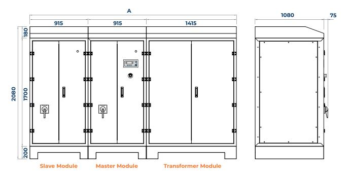
• 500kVA | 600kVA - A= 2745mm (Transformer Module (same size as slave module) + Master Module + Slave Module)
