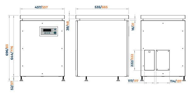
Dimensions for 450 enclosure • 10-15kVA (output 400Hz)
