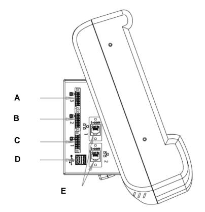
A – Serial Port (Optional Relay output)B – Serial Port (Optional Relay output)C – Relay OutputD – (2x) USB 2.0 PortE – (2x) Ethernet PortFigure 5Features available on left side of BloodTrack Kiosk V5
