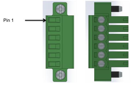
Figure 19 Lock connection—terminal block—pin 1 at top
