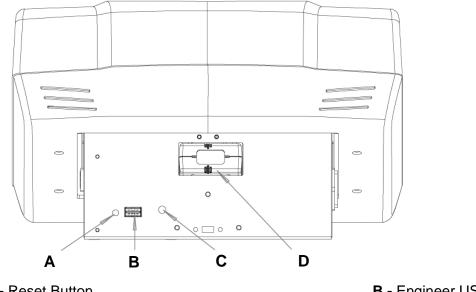
A - Reset ButtonB - Engineer USB portC - Emergency Access SwitchD - Barcode Reader
