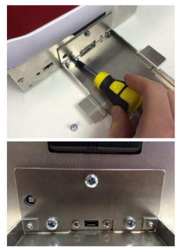
Figure 8 Assembling active shelf—affixing shelf chassis with screws to BloodTrack Kiosk V5
