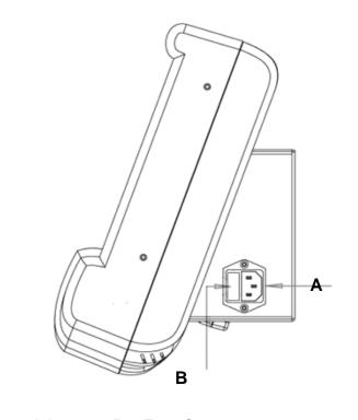
A – Latching Power InletB – Fuse CaseFigure 4Features available on right side of BloodTrack Kiosk V5
