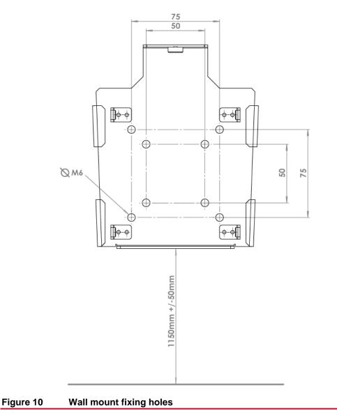
4. Once the wall mount is secured appropriately, attach the kiosk bracket to the back of the BloodTrack Kiosk V5 using four M4 x 10 screws.
