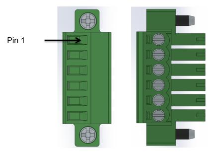
Figure 19Lock connection—terminal block—pin 1 at top
