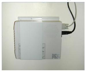
Figure 18 UPS mounted below Kiosk V5
