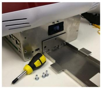
Figure 7 Assembling active shelf—aligning shelf with holes on Kiosk V5
