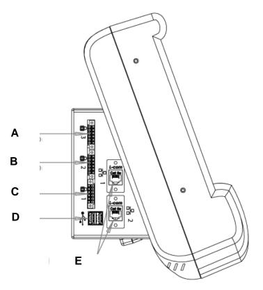
A – Serial Port (Optional Relay output) B – Serial Port (Optional Relay output)
