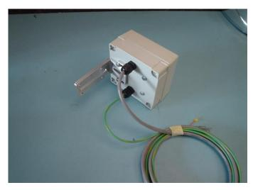
Mounting bracket on rear of electromagnet and two cables—signal and protective earth
