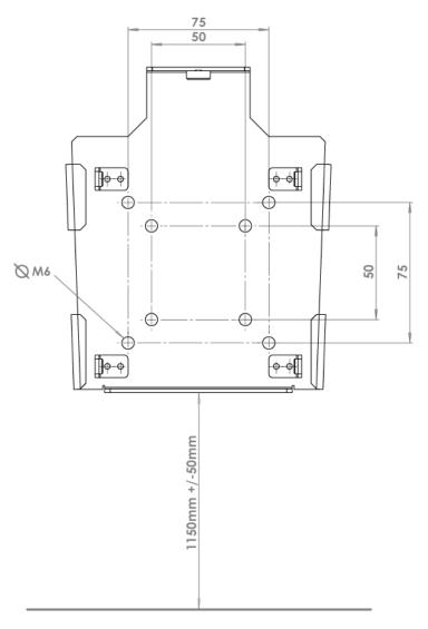
Figure 10 Wall mount fixing holes
