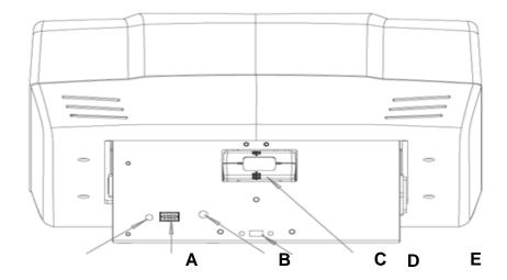
A - Reset button B - Engineer USB port C - Emergency Access Switch
