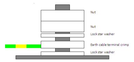
Figure 17 Electromagnetic lock—connection to earth point
