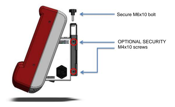
Figure 13 Securing wall mount
