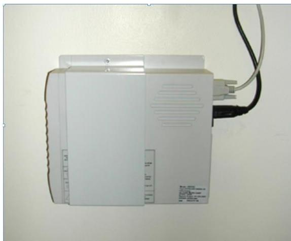
**Figure 18** UPS mounted below BloodTrack Kiosk V5
