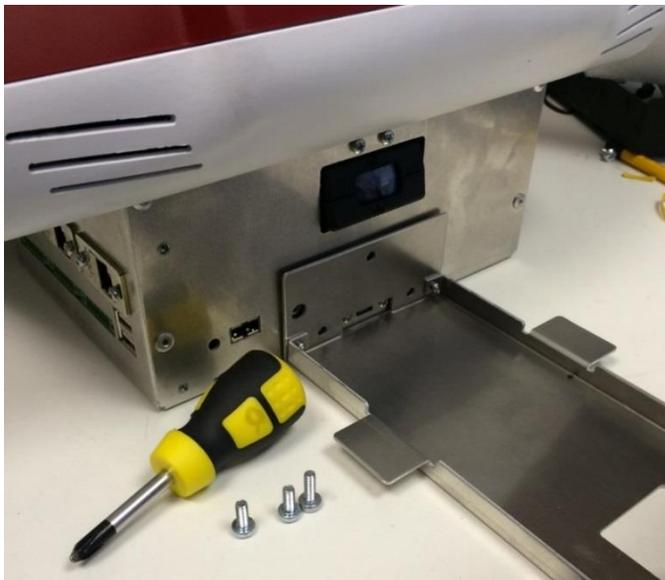
**Figure 7** Assembling active shelf—aligning shelf with holes on BloodTrack Kiosk V5
