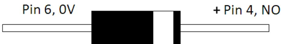
**Figure 20 Fitting diode to powered magnetic lock**
