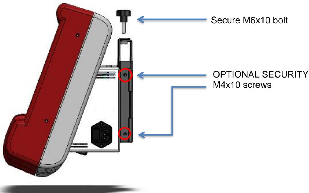
**Figure 13**      **Securing wall mount**
